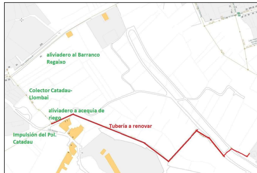
Fig.1. Colector a renovar
