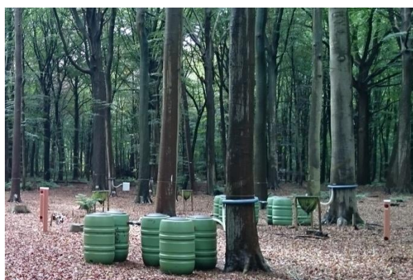
Figure 5-1: Throughfall and stem flow collectors on Level II plot in Wijnendale forest, Belgium.
