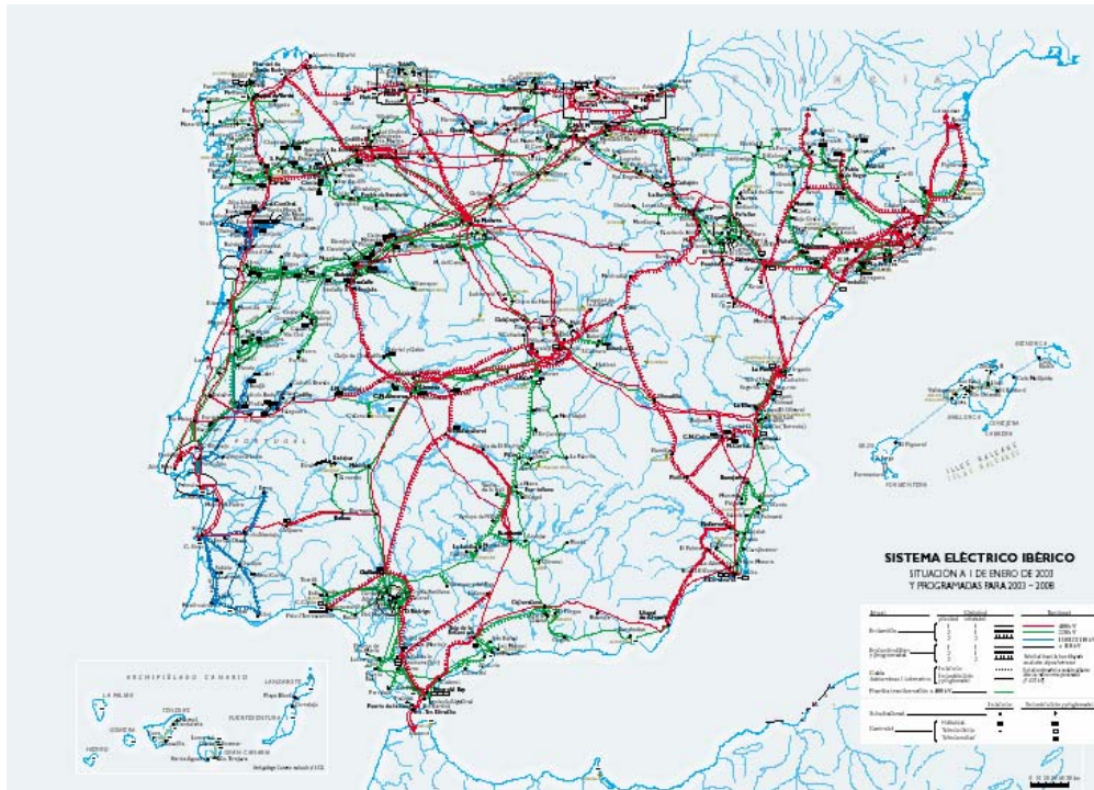
Fig. 13.12. Electric energy transport network. Source: REE.
