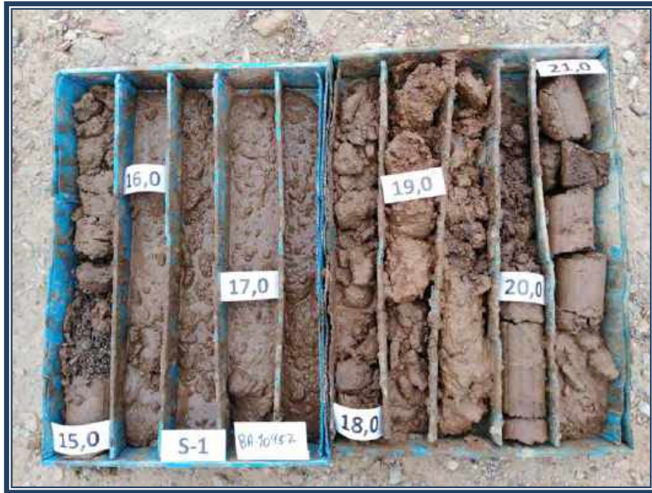
CAJAS DE TESTIGOS DEL SONDEO PZ-1 15,0 – 21,0 m
